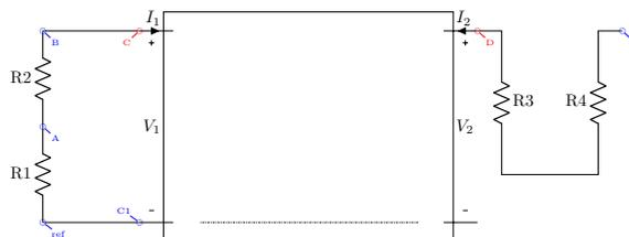
Fitting some circuit inside the Quadripole (nodes C and E):
